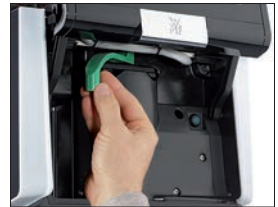
Rotate the lock by 180°
